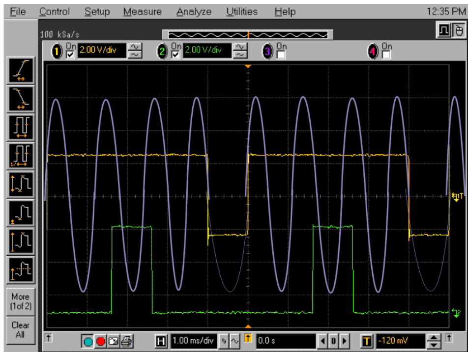
Figure 8-3 Viewing the Gate Timing with an Oscilloscope
